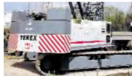
Counterweight hydraulically extends
