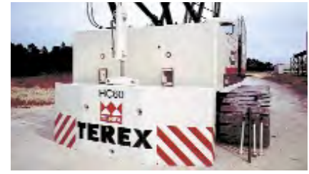
Hydraulic removable counterweight system
